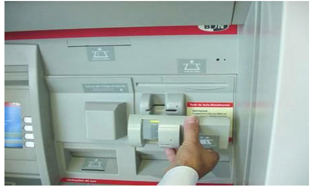
Equipment being installed on front of existing bank card slot.
