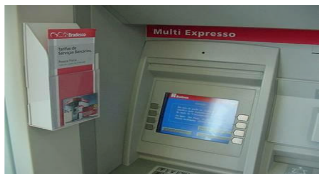
The PIN reading camera being installed on the ATM is housed in an innocent looking leaflet enclosure.
