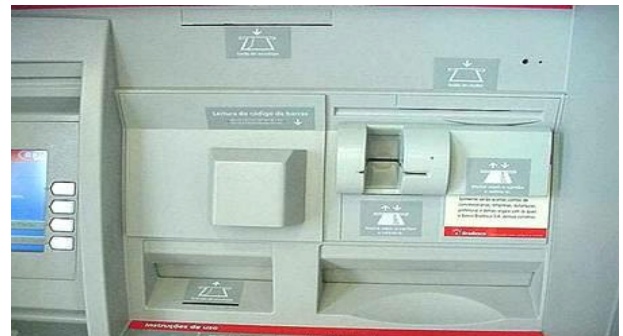
The equipment as it appears installed over the normal ATM bank slot.
