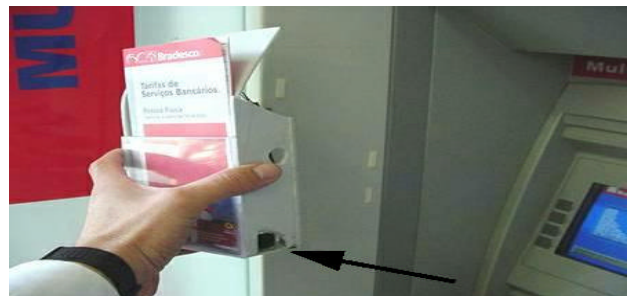
The PIN reading camera being installed on the ATM is housed in an innocent looking leaflet enclosure.
